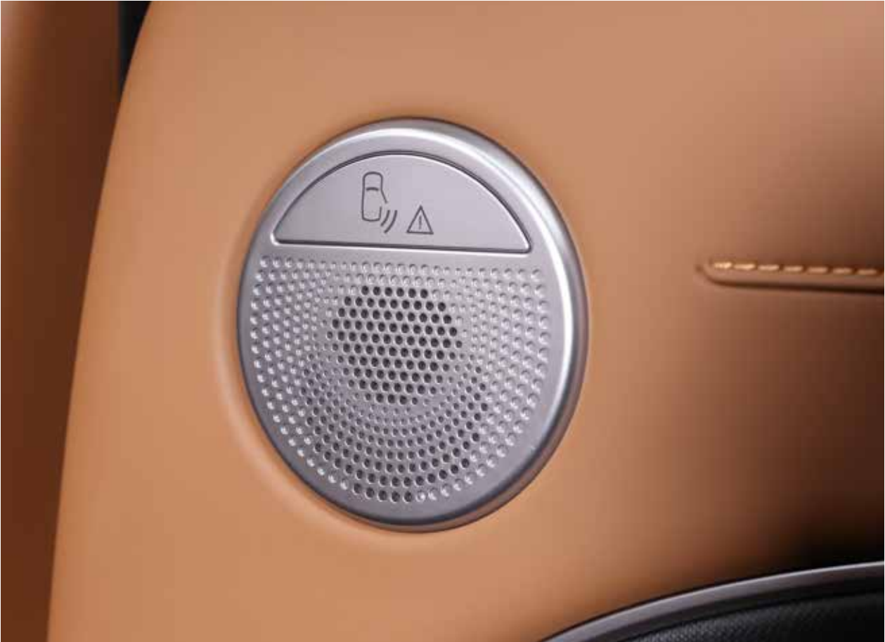
Safe Exit Warning
